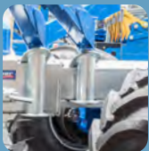
Telescopic frame, adjustable after the 1. stanchion bench
